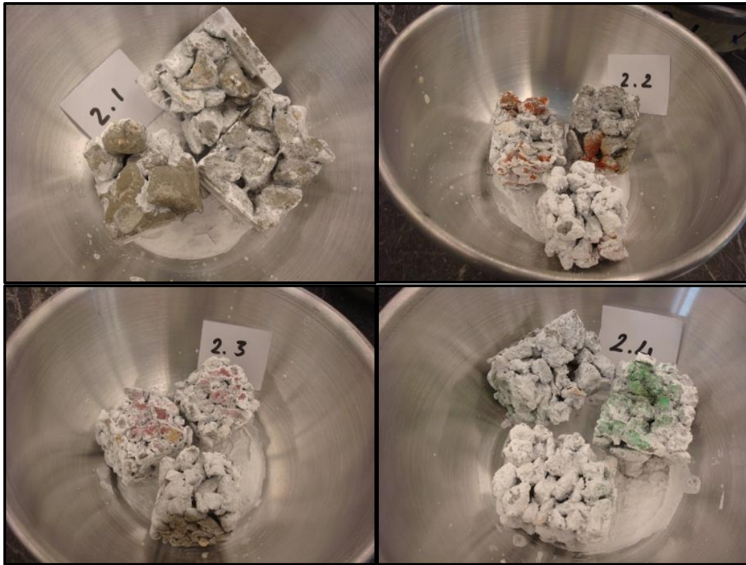
Figure 4.34 Specimens for 350 kg cement mixtures after soaking in salt
