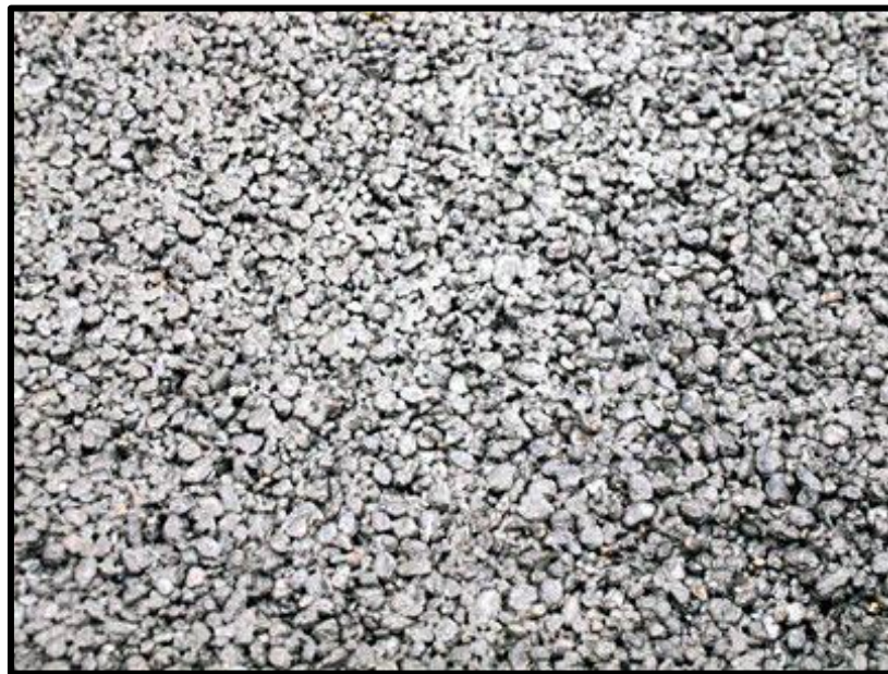
Figure 1.1 Texture of pervious concrete (NRMCA, 2011)
