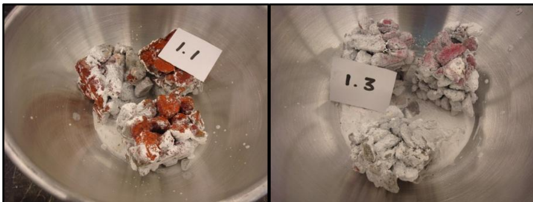
Figure 4.33 Specimens for 250 kg cement mixtures after soaking in salt
