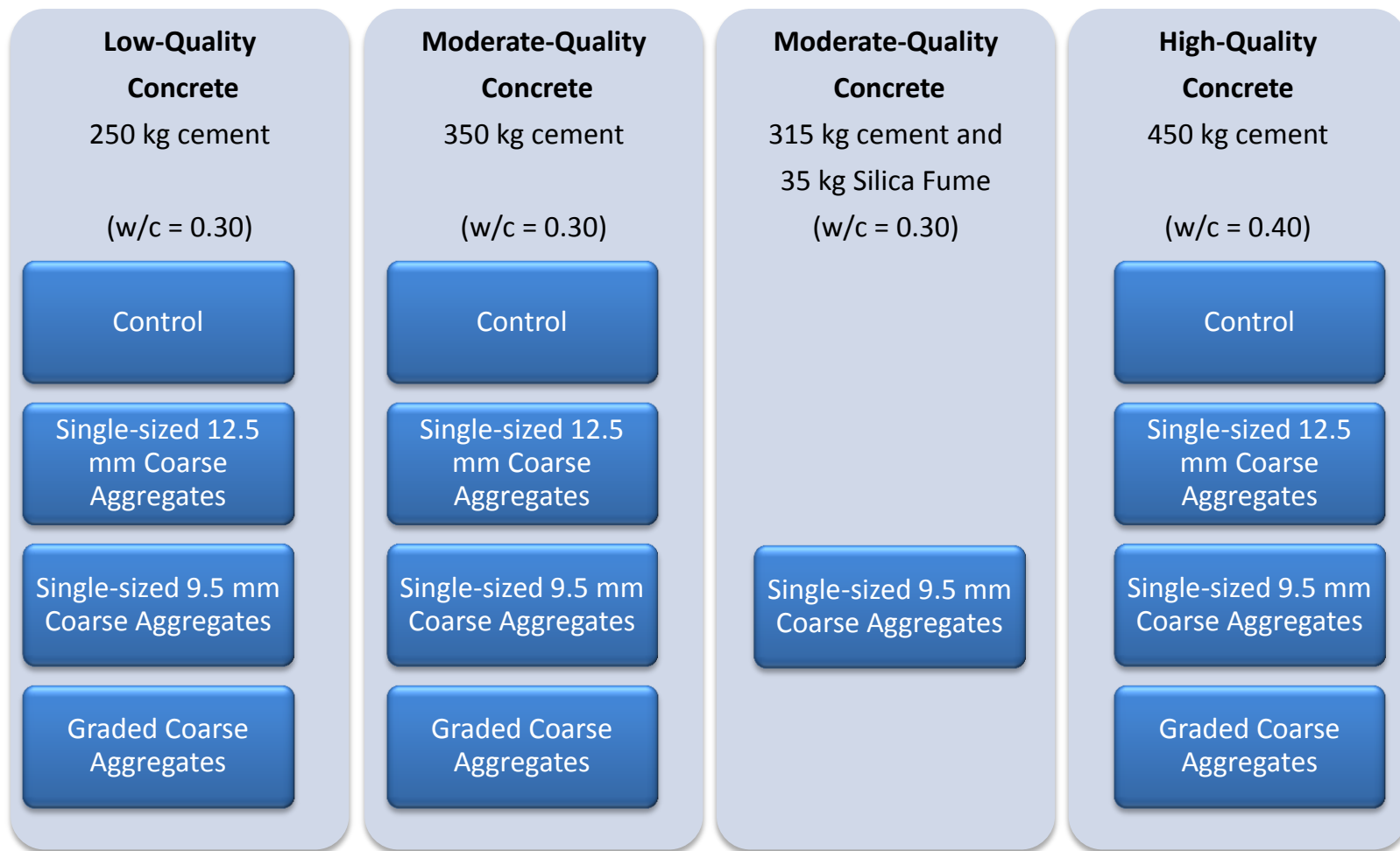
Figure 3.1 Breakdown of concrete mixtures prepared
