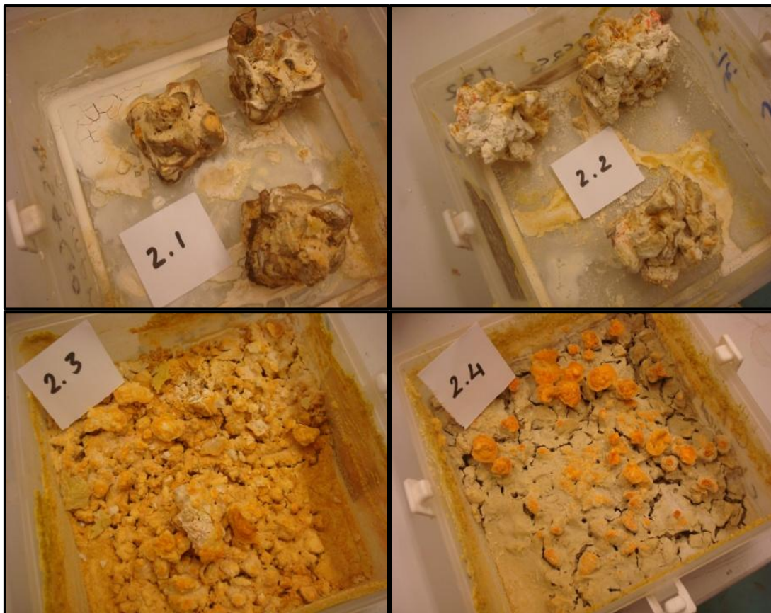
Figure 4.29 Specimens for 350 kg cement mixtures after soaking in acid
