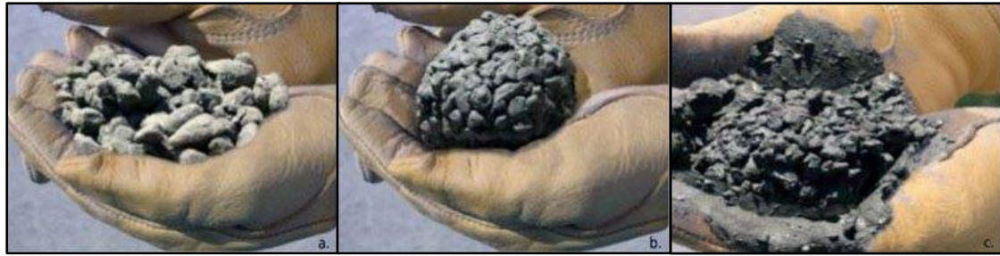
Figure 2.4 PCPC water content (a) too little water, (b) proper amount of water, and (c) too much water (NRMCA, 2011)
