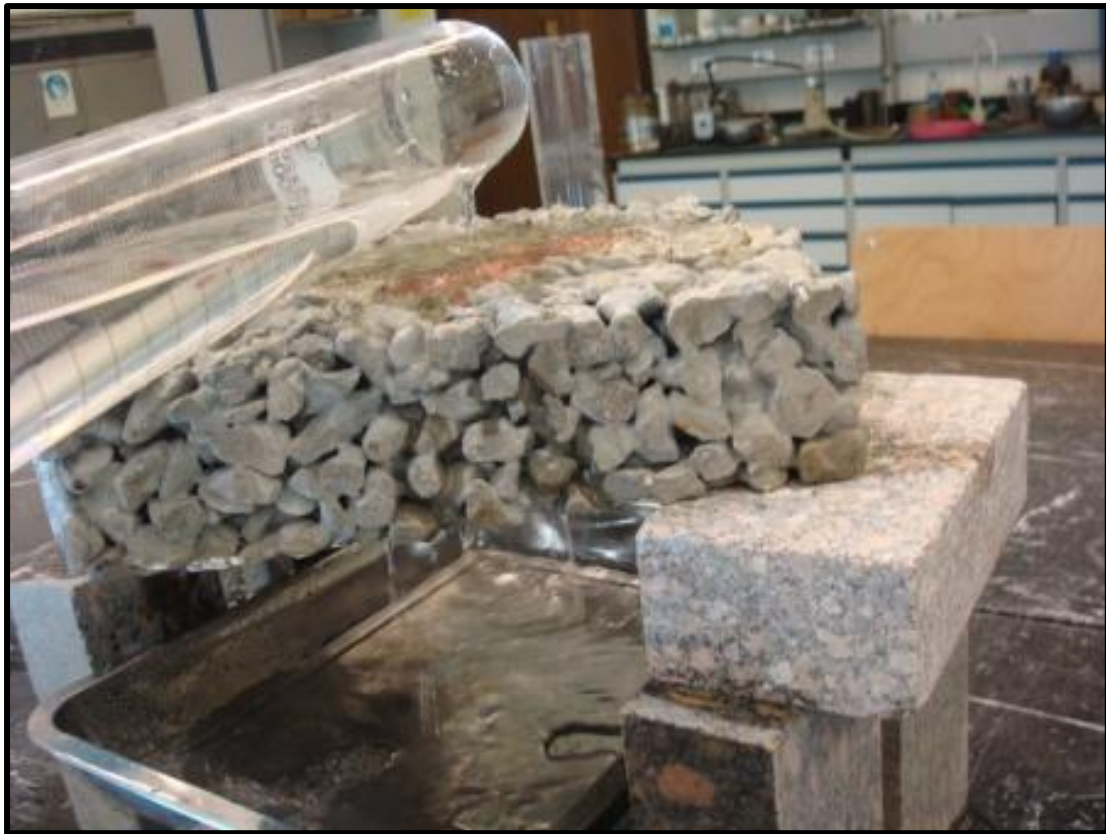
Figure 4.45 Water seeping through sides of the sample
