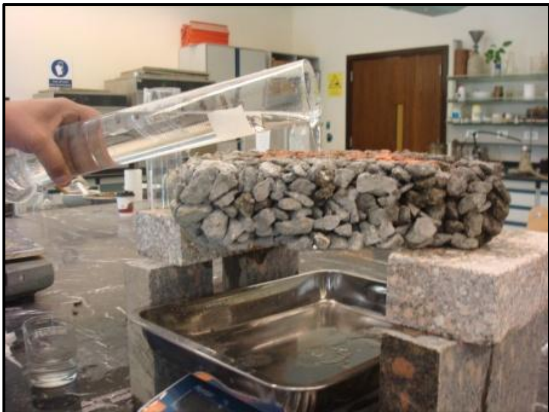
Figure 4.40 Experimental procedure designed to study permeability of PCPC
