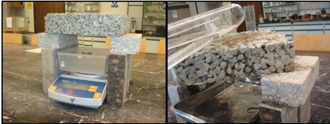
Figure 3.16 Apparatus designed to measure permeability
