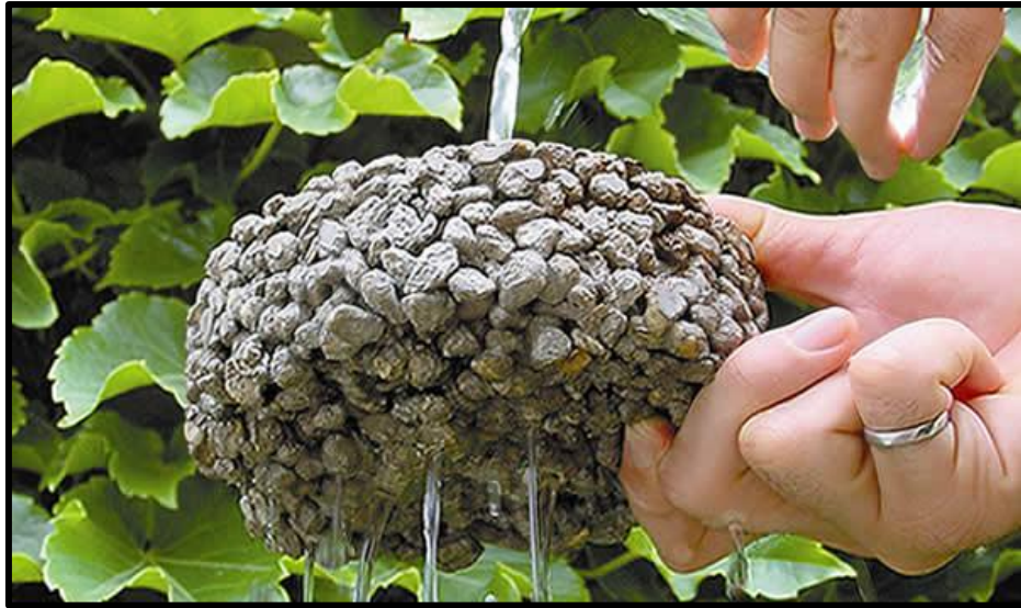
Figure 1.2 Pervious concrete draining water (NRMCA, 2011)
