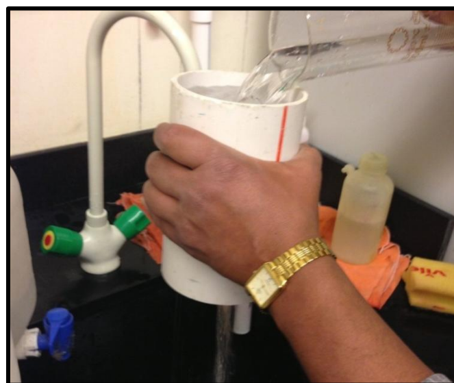
Figure 3.18 Washing the specimen
